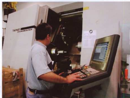
State-of-the-art technology in all areas One of CDL Präzisionstechnik's 40 CNC high-performance processing machines with twin heads
