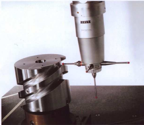
CDL Präzisionstechnik's axial control curve technology produces parts that don't require any work after the heat processing
